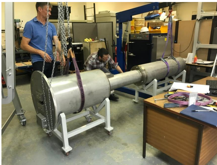
Figure 7. Photograph of the flight tube during assembly. The rear flange is to the left of the photograph.
