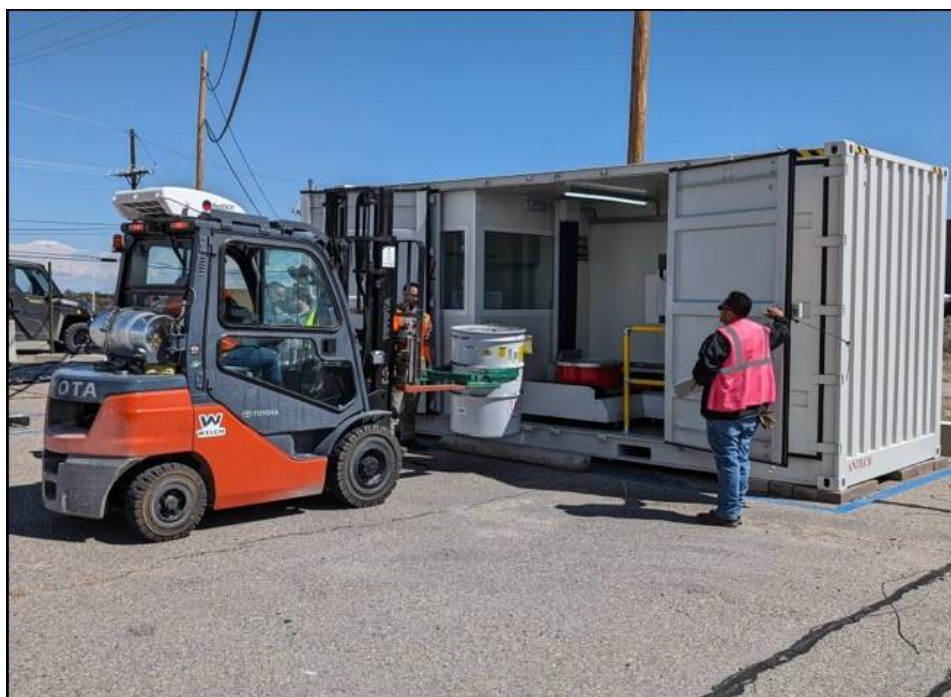
Fig. 2. The UDASS in operation in Area G of TA-54 at LANL. The photograph shows a TRU waste drum being loaded into the UDASS for measurement.
