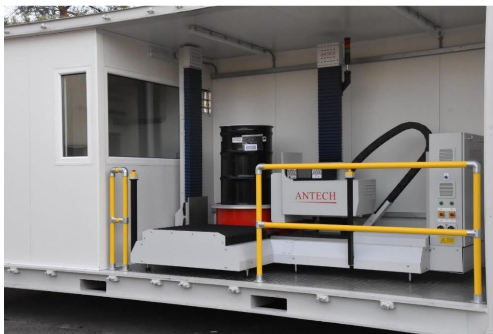
Fig. 1. UDASS mounted in an ISO shipping container. The operator control room is shown on the left. The photograph shows the UDASS mobile lab with a drum in the measurement position and the foldable side doors open.
