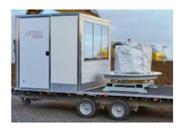
CHARMS employs the Far Field measurement method, viewing the entire waste object (drum, waste bag) being measured. Using the weight measured by the load cells in the turntable (rotation platform) an average density attenuation correction is performed. During each measurement the waste object (for example drum or waste bag) is rotated at a constant rotation speed to reduce the effect of inhomogeneity in the waste matrix.
