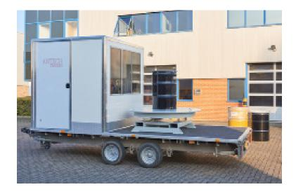
CHARMS is designed to operate on 110 VAC, which may be supplied from 110 VAC mains or 240 VAC mains (through an isolation step-down transformer) or by on-board portable generator.
